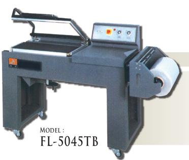
L-Type sealing knife achieves sealing one time. TEFLON non-adhesive layer, non-adhesive sealing film result in sealing neat and without splitting. After sealing, materials will be transmit into tunnel to shrink automatically.
